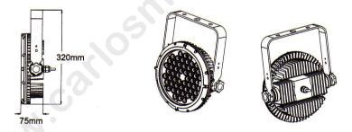
For improving the waterproof grade, Our company provides another mode the head can separates from the lighting. If the lighting needs to work in the water for a long time, you should choose and buy this mode, such as the above figure. The waterproof grade of the head reaches IP68.
