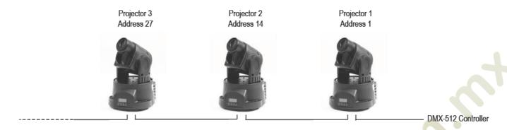
The wires must not come into contact with each other, otherwise the fixtures will not work at all, or not will work properly.
