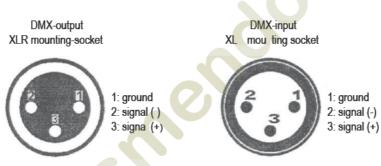
If you are using controllers with this occupation you can connect the DMX-output of the controller directly with the DMX-input of the first fir ture in the DMX-chain. If you wish to connect DMX-controllers with other XLR-outputs, you need to use adapter-cables.
