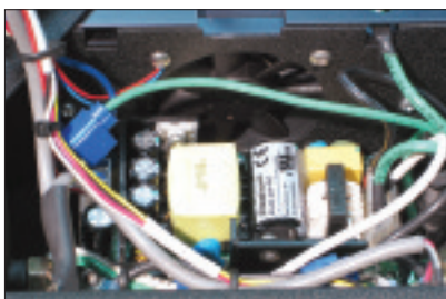
Fig. 13: Power supply and fan.
