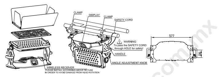
Take 2 clamps and safety cord out from the package and mount 2 clamps on the underside of fixture with 2 retainers attached to each clamp. Hang the fixture on the structure and fasten the screws attached to each clamp. Always ensure that the projector is firmly anchored to avoid vibration and slipping whilst functioning. Always ensure that the structure that you are going to mount the projector is secure and is strong enough to support a weight of PR-8800. **WARNING:**
