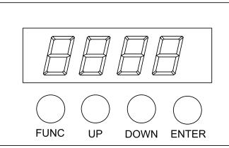
Projector configuration can be set conveniently via push-button switch and LED display.
