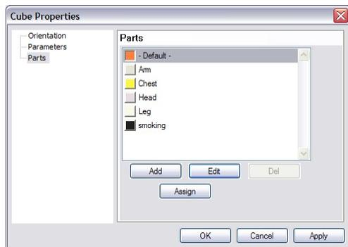
The parts page allows you to manage parts in this object. All primitive used in the open object belong to a part. All primitives belonging to the same part have the same color or material.
