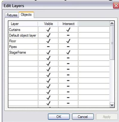
In this dialog, you can edit the object layers. You can edit the name of a layer by clicking in the left box (layer line will become active), and then clicking in it again. You can then edit the existing name or enter a new name. In the 'Visible' column, you can select which layers are visible (' ✓ ') or hidden (' - '). The 'Intersect' column determines if beams are projected on the objects contained in the layer or will pass through.
