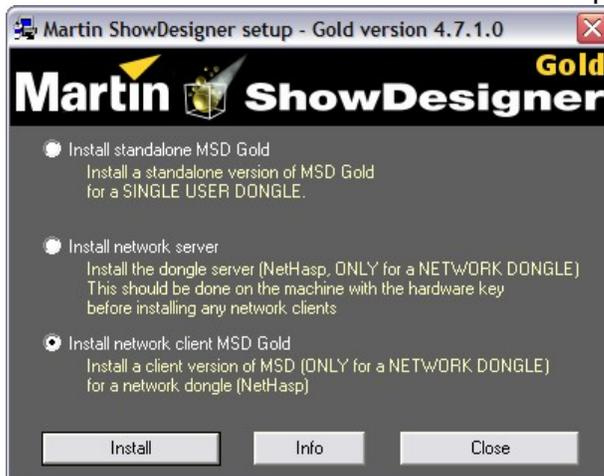
Install a client version of MSD (only for a Network Dongle) on machine(s) on the same network as the MSD Network server.
