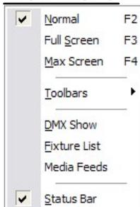
You can use the entries in this menu to select the screen mode or to view or hide the toolbars holding the buttons, the DMX show window and the status bar at the bottom of
