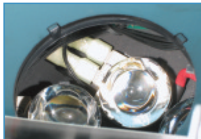
Figure 3 - LED and connections
