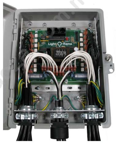
13. This completes the assembly of your controller. (Note that this picture shows the fuse covers – these were a late addition designed to protect the wires passing over the fuses.) You are ready to configure it for testing.
