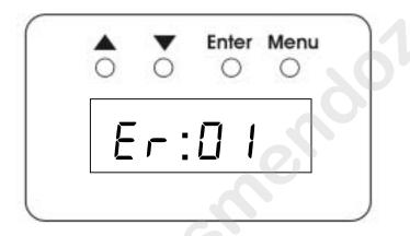
Error 01 is displayed for an overtemperature condition. Error 02 is displayed for an overvoltage condition.
