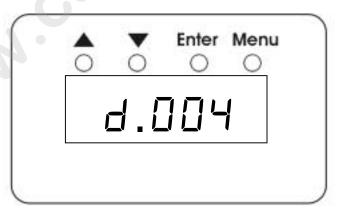
The UP/DOWN keys change the value for the start address. The ULD-360 uses the changed value immediately and permanently saves it after 10 seconds or if the Enter or Menu key is pressed.
