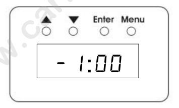
Once the input levels for all dimmer channels have been shown, the display will then indicate the output level for each channel. This is indicated by the letter 'o' in the display, followed by channel number, followed by output level. Output will be shown as a percentage, with 100% indicated b the letters 'FF'
