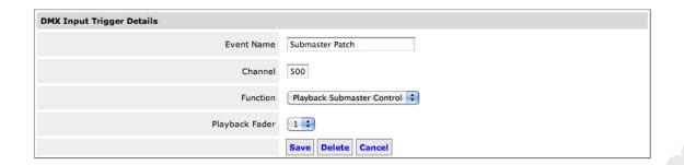
In this example, the DMX Input trigger has been configured to take the input level of Channel 500 and use it to automatically adjust the submaster level of Playback 1.
