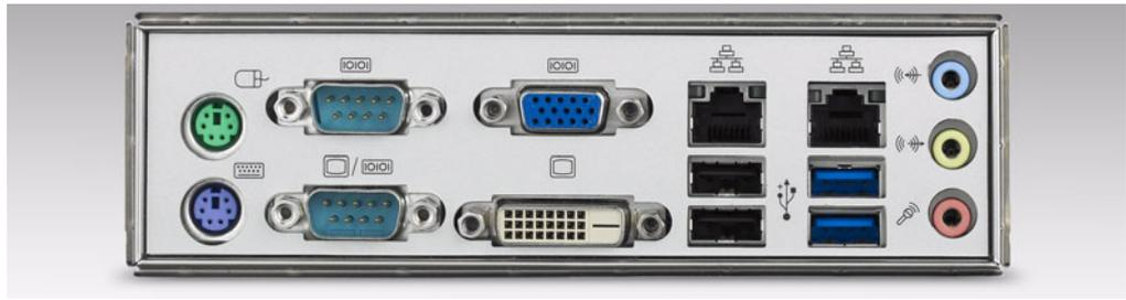
Figure 1.2 I/O Connectors
