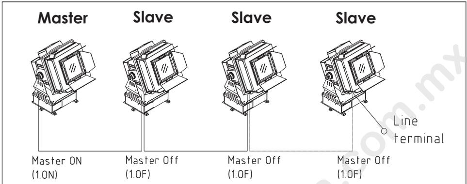
The line terminal is a resistor fitted between the 2 Signal Pins (2 and 3) at the end of the DMX line. This is to avoid the defective functioning of the DMX line. A 120 Ohm resistor is suggested.
