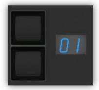
There are 2 separate sets of page control buttons, one for the Playback Faders and another for the Matrix buttons. Paging essentially gives you additional virtual sets of faders and matrix buttons to work with. Paging can be controlled by your lighting software or by the MIDICON-2<sup>TM</sup> controller via MIDI channel paging. If your software can control the paging you can have up to 99 pages to work with.
