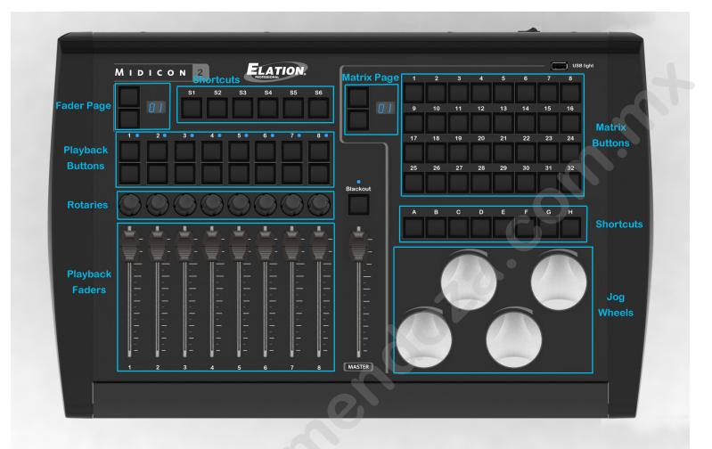
**PLAYBACKS:** 8 playback faders each with 1 rotary push-in style dial, 2 playback buttons with bi-color LEDs, up and down fader page select buttons, and an LED page number display
