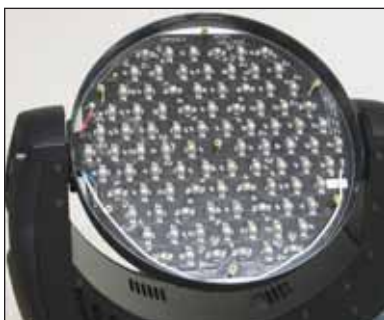
Fig. 4: LED array without lenses
