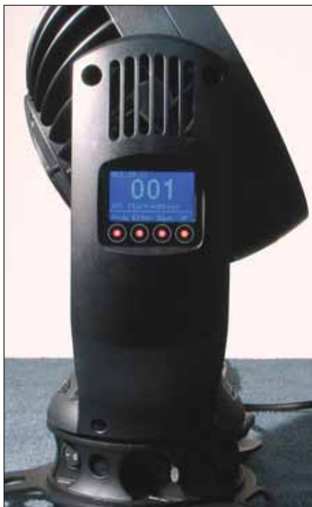
Fig. 15: Yoke arm and display
