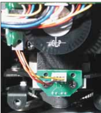
Fig. 9: Tilt encoder and pan gear
