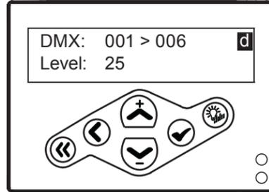
The two LEDs on the user interface indicate power and DMX signal. When power is applied, the blue "Power" LED is illuminated. The green LED indicates DMX signal. When no DMX signal is present, the green LED will flash. When a stable DMX signal is present, the green LED will illuminate fully.
