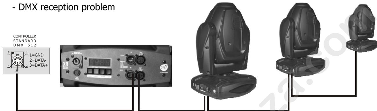
For Installations where long distance DMX cable connections are needed, we suggest to use a DMX terminator.
