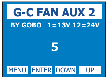
GOBO-COL. FAN SPEED WHEN GOBO WHEEL INSERTED
