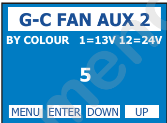
GOBO-COL. FAN SPEED WHEN COLOUR WHEEL INSERTED
