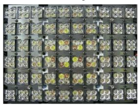
Apply the new lenses set on top of the frotal LEDs panel with 12° lenses and tighten again the 4 screws previously removed
