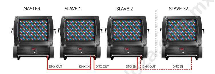
To activate Auto mode on the first unit, use the menu to run through the different modes until AUTO appears on the display, and press enter.
