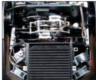
Fig. 5: Lamp house and optical assembly
