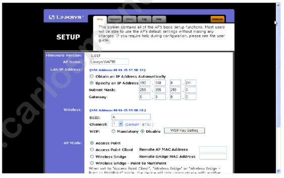
Here it can be seen that this WAP has its SSID set to A and its Channel is set to 1. If the SSID of the Tubes are also set to A then the system will work and the encoder Tube will route its airborne DMX data via the WAP, if there is any discrepancy it will not work, please note the SSID is cAsE SeNsItIvE.
