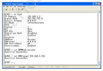
Again at this stage it is imperative to save the config to non volatile memory using the "save conf" command
