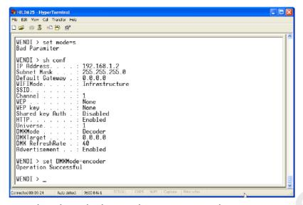
Now that the Tube knows that it is an encoder it is important to set the target address so that the Tube knows where to send the data.
