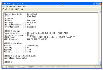
It is now imperative that you save the configuration of the Tube at this stage, otherwise when you reboot the Tube the IP address change will be forgotten.
